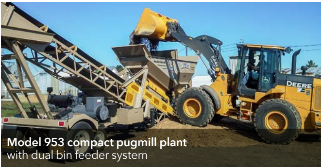
PLC control system allows for precise metering of materials to the pugmill plant
