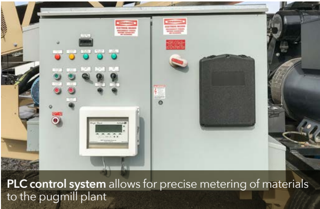
Model 953 compact pugmill plant with dual bin feeder system
